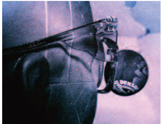
Figure 6. ANSI Z87 spectacle failure with squash ball at 90mph
