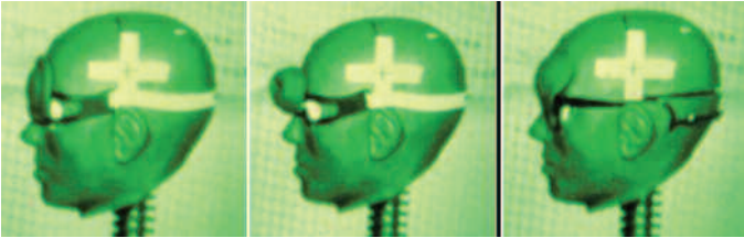
Figure 17. Racquetball eyeguard testing for ASTM F803 (1983)
