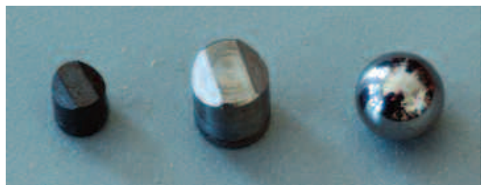
Figure 7. Military fragment simulators and ANSI High velocity test object
