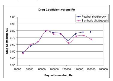
Fig. 2. Comparison between standard feather and synthetic shuttlecocks
