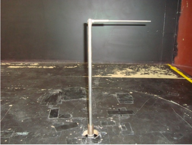
Figure 5. Wind tunnel testing of shuttlecock (experimental rig only)
