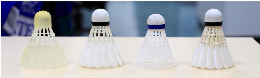
Figure 3 (L-R) Shuttlecock model fabricated by additive manufacturing, Mizuno NS-5 synthetic shuttlecock, regular synthetic shuttlecock and traditional feather shuttlecock.
