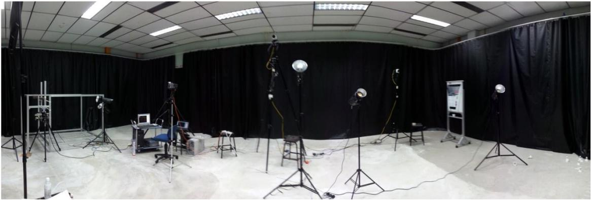
Figure 80 Experimental setup for trajectory capture of the shuttlecocks.
