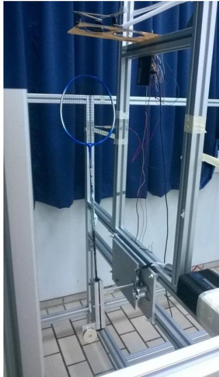
Figure 111 The extended badminton racket for attaining the desired smash speed.
