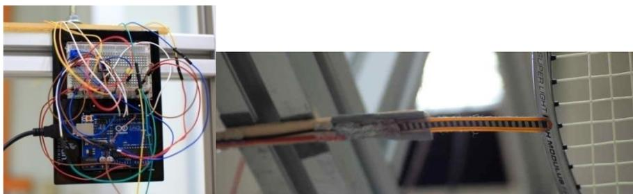
Figure D3 L-R Arduino circuit board with the prototyping breadboard. Flex resistor to determine the racket position.
