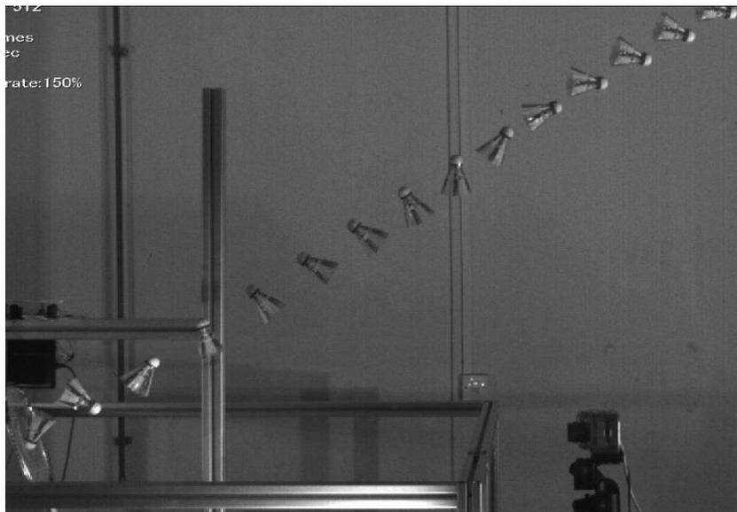
Figure 83 Turnover behaviour observed from one of the runs of the Yonex Mavis 350 shuttlecock.
