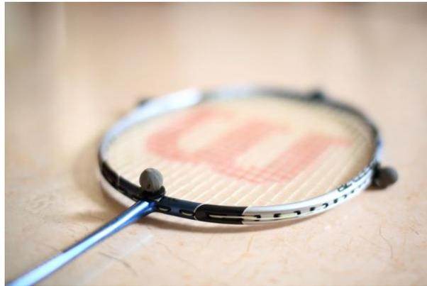
Figure 74 Motion tracking markers on the badminton racket.
