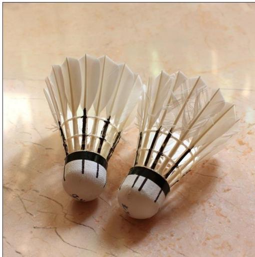
Figure B3 Typical damage of 3-5 feathers in one launch using a launcher, in contrast to a perfect condition shuttlecock.
