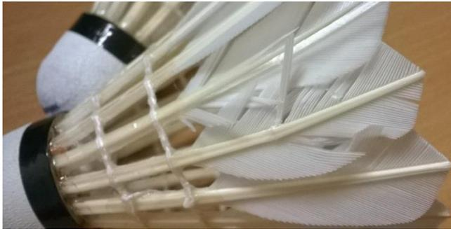
Figure 104 (L) Feather vane wear from usage.
