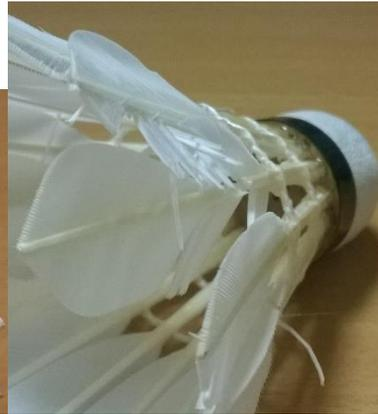
Figure 105 (R) Feather shaft breakage from usage.
