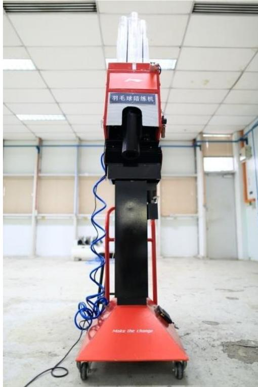
Figure B2 Compressed air driven badminton shuttlecock launcher used for the experiment.
