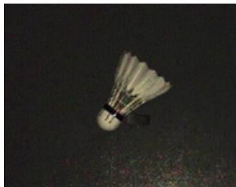
Figure 54 The markings drawn on the shuttlecock for determining spin rate in post-experiment video processing.
