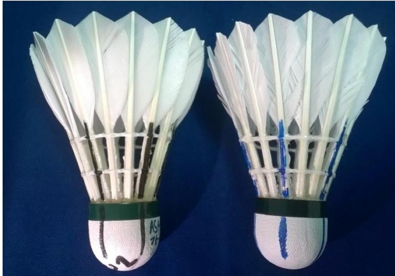
Figure 131 Feather vane condition of the Yonex AS40 (left) and Li-Ning A62XD (right) after 15 smashes.
