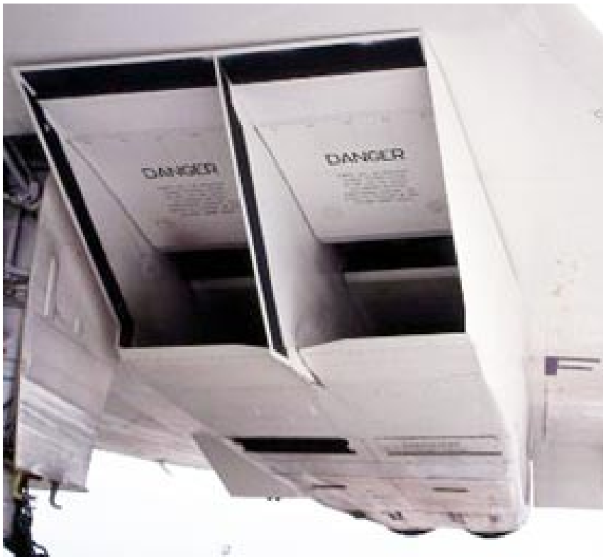
Air intake of a Concorde
